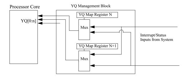
If interrupt request signals are brought into the YIELD qualifiers as described, even an interrupt condition that is masked by software so that it will not cause any exception vector to be executed can be used to enable the rescheduling of a service thread, for "zero latency" handling. On processors and VPEs using fine-grained multithreading, this has the additional advantage of not causing the processor/VPE to suspend multithreading due to entry by one thread into an exception handler.
